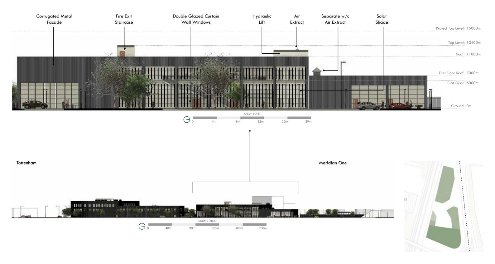
Project Summary: With the main aim of this proposal being to bridge the gap between 2 communities, the project's external cladding connects with the surrounding area's typology (Industrial warehouses) with corrugated metal sheet panels. Elevation: This drawing was made using Autodesk Revit and Photoshop to highlight the buildings cladding, size and height in relation to its surrounding area. Additionally, how users would interact with the proposal internally and externally.
